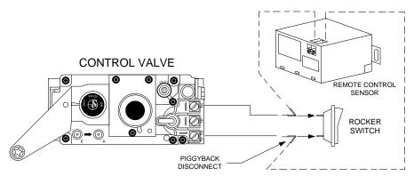
Remember the Rocker Switch must be turned to "OFF" while using the Remote Control.
